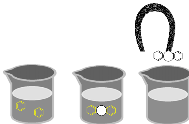
Figure 16. Magnetic extractants used to remove 99.995% of the benzene originally present in a sample of water (left). The extractant contains a non-polar group that binds to the contaminant (middle), and the extractant and the bound contaminant are then removed using a magnet (right).
